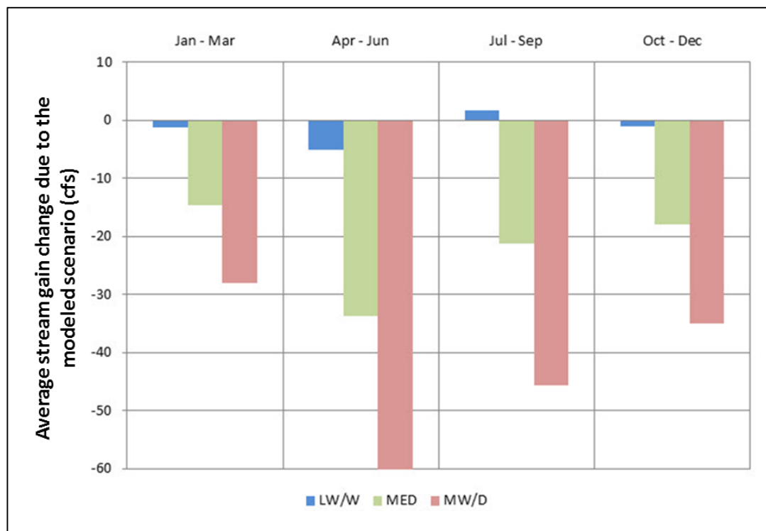
Figure 33 Baseflow change due to the climate change conditions, increased pumping scenario.
